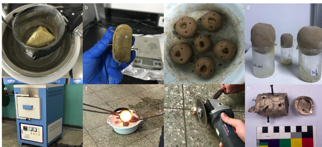
Figure 1 Procedure used for the direct lost-wax casting in this experiment
