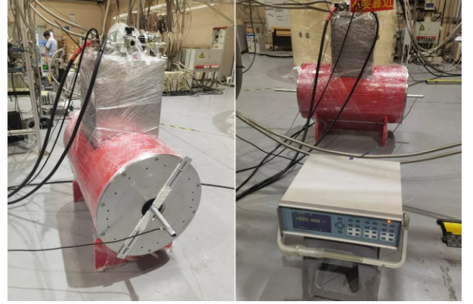
Figure 6. Superconducting solenoid magnet system. After undergoing training quenches, it achieved the design current of 240 A, offering a uniform magnetic field of 7 Tesla within a central air region of \phi 40 \text{ mm} \times 600 \text{ mm} .
