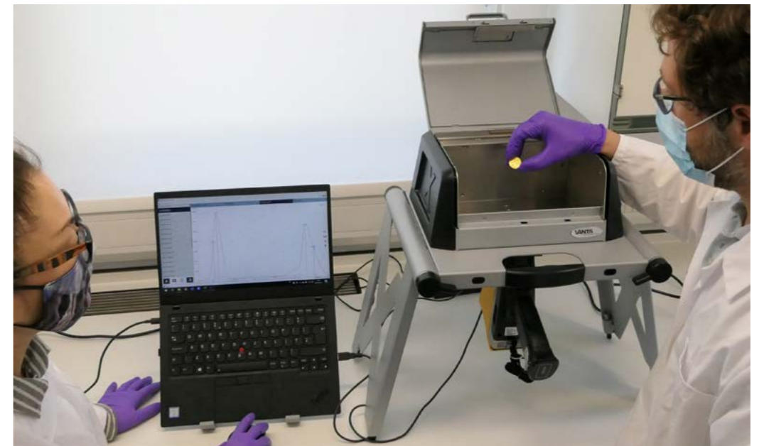
Figure 2: Placing a gold coin in a secure chamber for benchtop pXRF.
