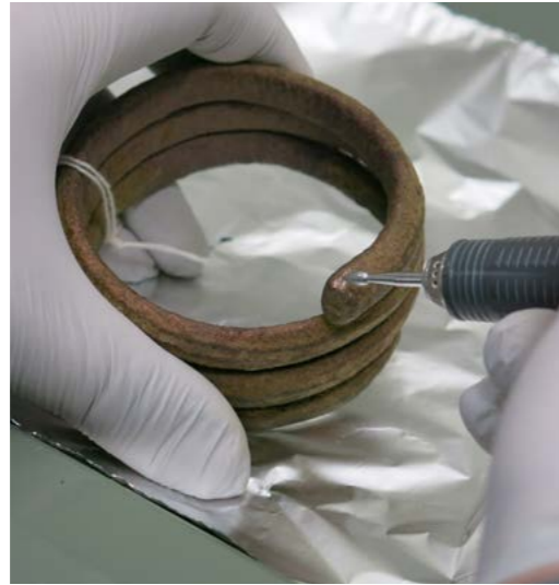
Figure 5: Using a rotary tool to remove the patina in a small spot of a metal object, to facilitate pXRF analysis.
