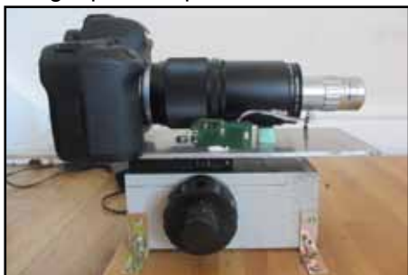
Fig. 1. The rail based on an old microscope.
