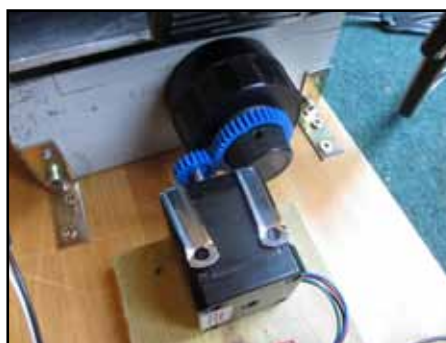
Fig. 4. Plastic gears driving the fine focus knob.
