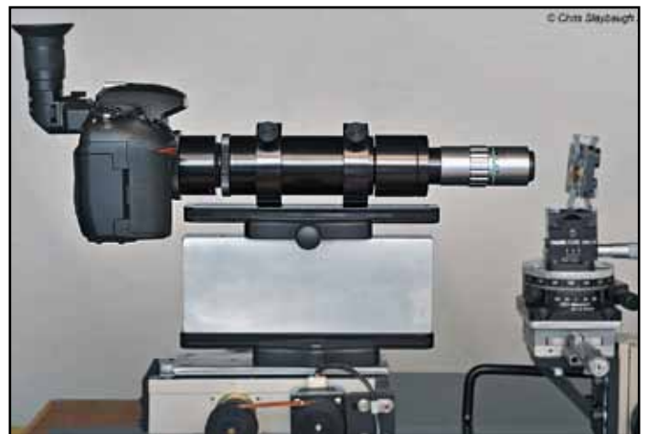
Fig. 20. The 'Bratcam' on which our system is based.
