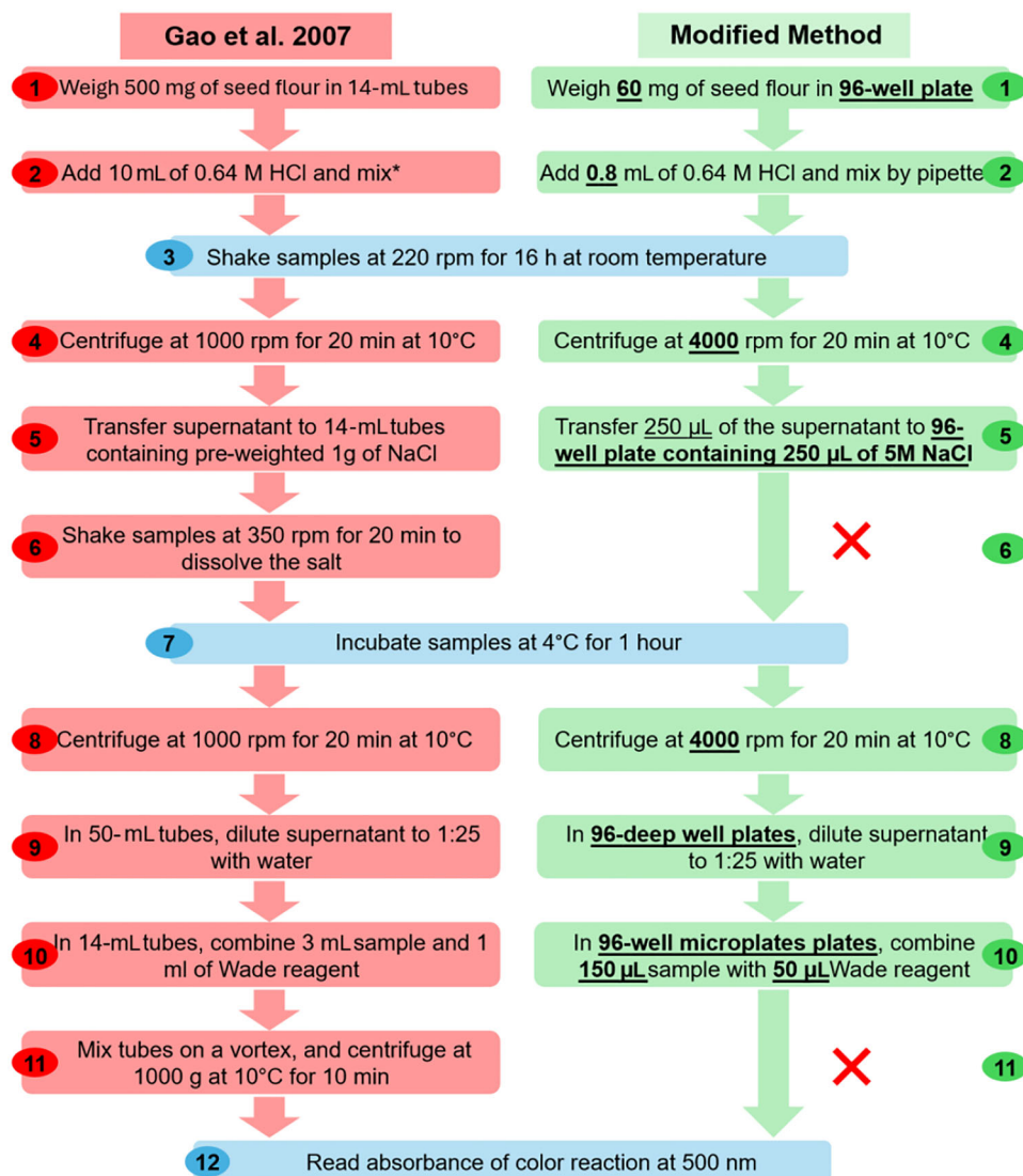
FIGURE 1 A step-by-step comparison of the original protocol by Gao et al. (2007) and the modified high-throughput assay. In the modified method, omitted steps are indicated by a red “X,” while other modifications are shown in bold text. The asterisk in step 2 indicates that Gao et al. (2007) did not specify how the samples were mixed; therefore, we mixed the samples by vortexing.
