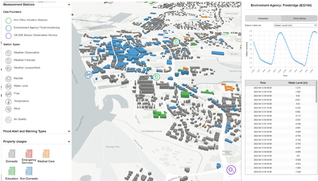
Figure 19. Consolidated visualisation. A built-in Visualisation Framework provides a uniform interface to retrieve and visualise data from TWA. It creates an aligned visualisation of previously isolated data sources side by side to foster fact-based decision-making and enable insights across domains.
