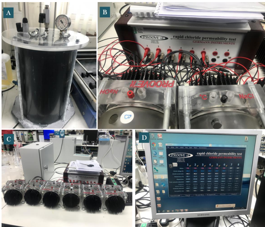
Figure 3.29 (A) Vacuum container; (B) reaction cells connecting with the power supply; (C) general setup and (D) Prove it software
