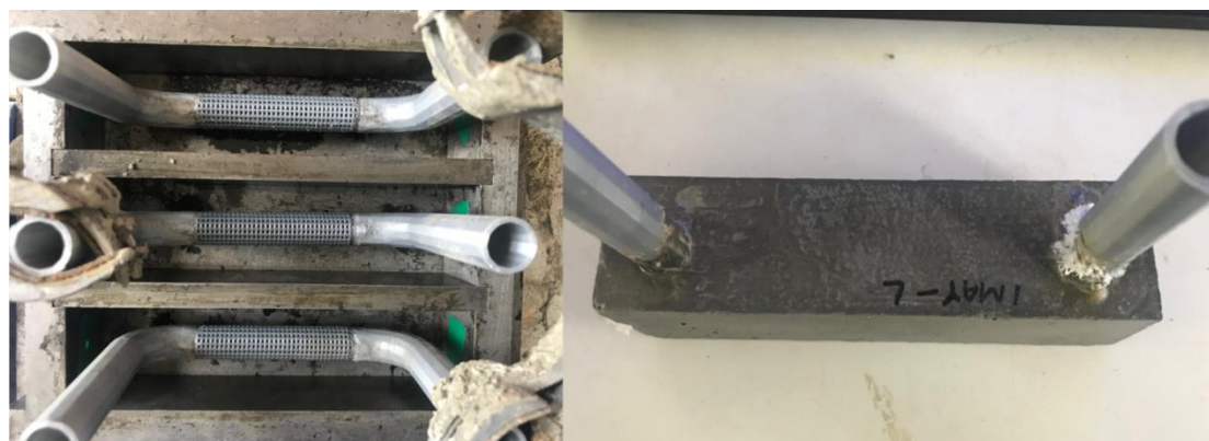
Figure 6.18 General set-up for cement casting (Left), and a cured beam after 7 days (Right)
