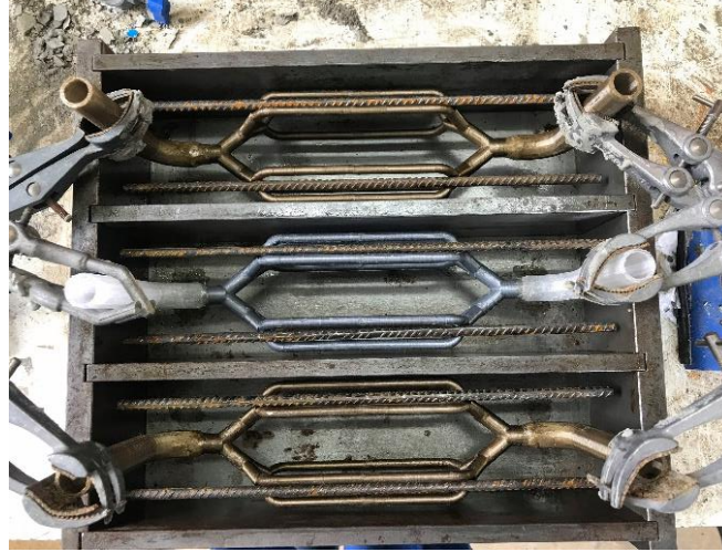
Figure 3.7 Set-up for PLA vascular system in mortar specimens
