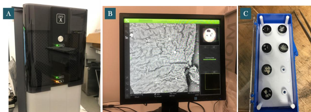
Figure 3.20 (A) Phenom® Pro G2 instruments for SEM-EDX analysis, and (B) analysis software and (C) sample prepare process
