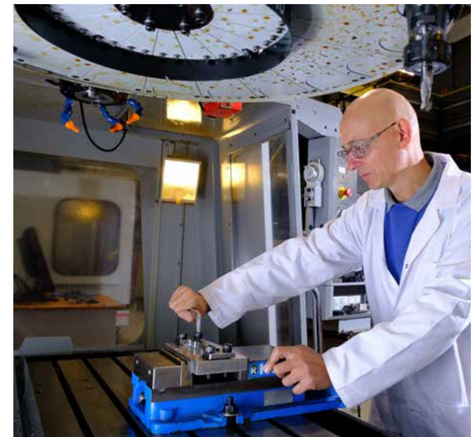
CNC machining, a technique used to manufacture moulds for injection moulding. Credit: University of Bradford
