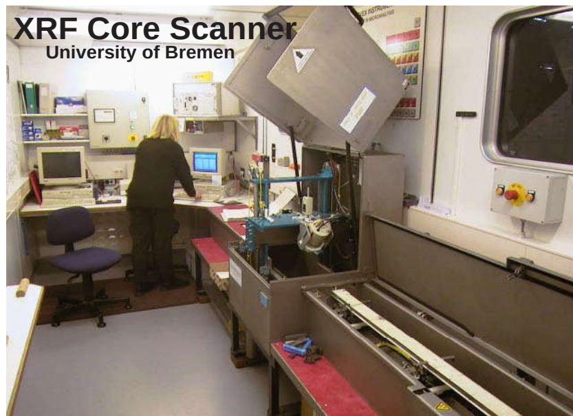
Figure 3.2: A photograph of the XRF Core Scanner of Bremen University that was used to obtain measurements for this study. On the right hand side a sediment core is visible. During operation the lid is closed, and the instrument visible along the centre of the right hand wall takes measurements. The computer equipment controls the operation of the instrument and is used for analysis.
