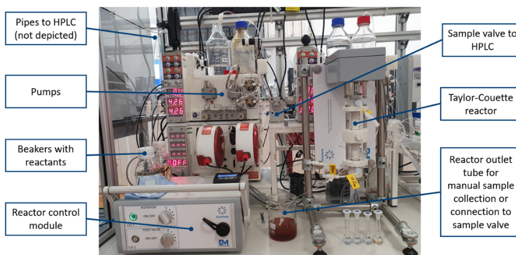
Figure 5: A labelled image of the experimental setup for data collection from Autichem's Taylor-Couette reactor.
