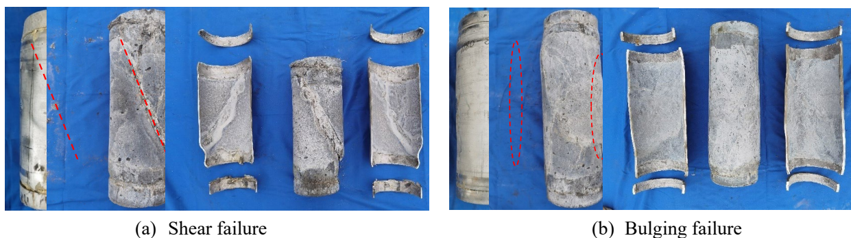
Fig. 7 Externally and internally observed failure of SS+UHPC column specimens
