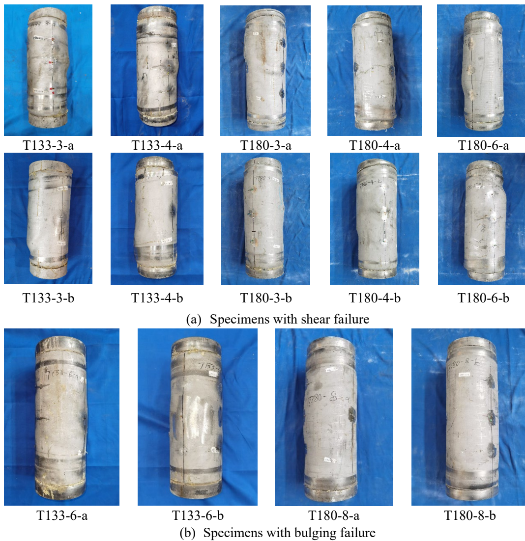
Fig. 8 Failure modes of all SS+UHPC column specimens
