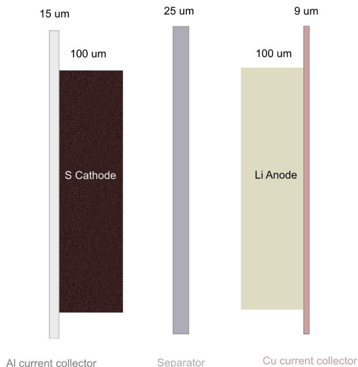
Figure 2.32 The Configuration of Li-S Batteries at Laboratory Scale
