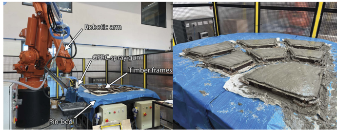
Figure 4. Digital fabrication setup (left) used to fabricate the sprayed GFRC conoid segments (right).
