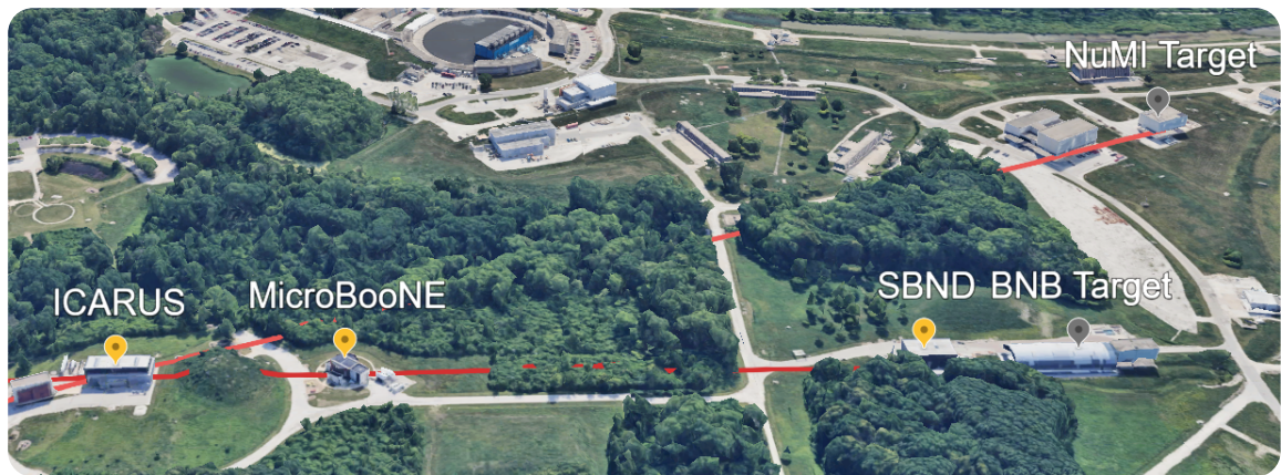
Fig. 5.1 Liquid-argon short-baseline detectors at Fermilab. The red line at the top illustrates the path of the NuMI beam starting from the target and the line at the bottom illustrates the BNB.
