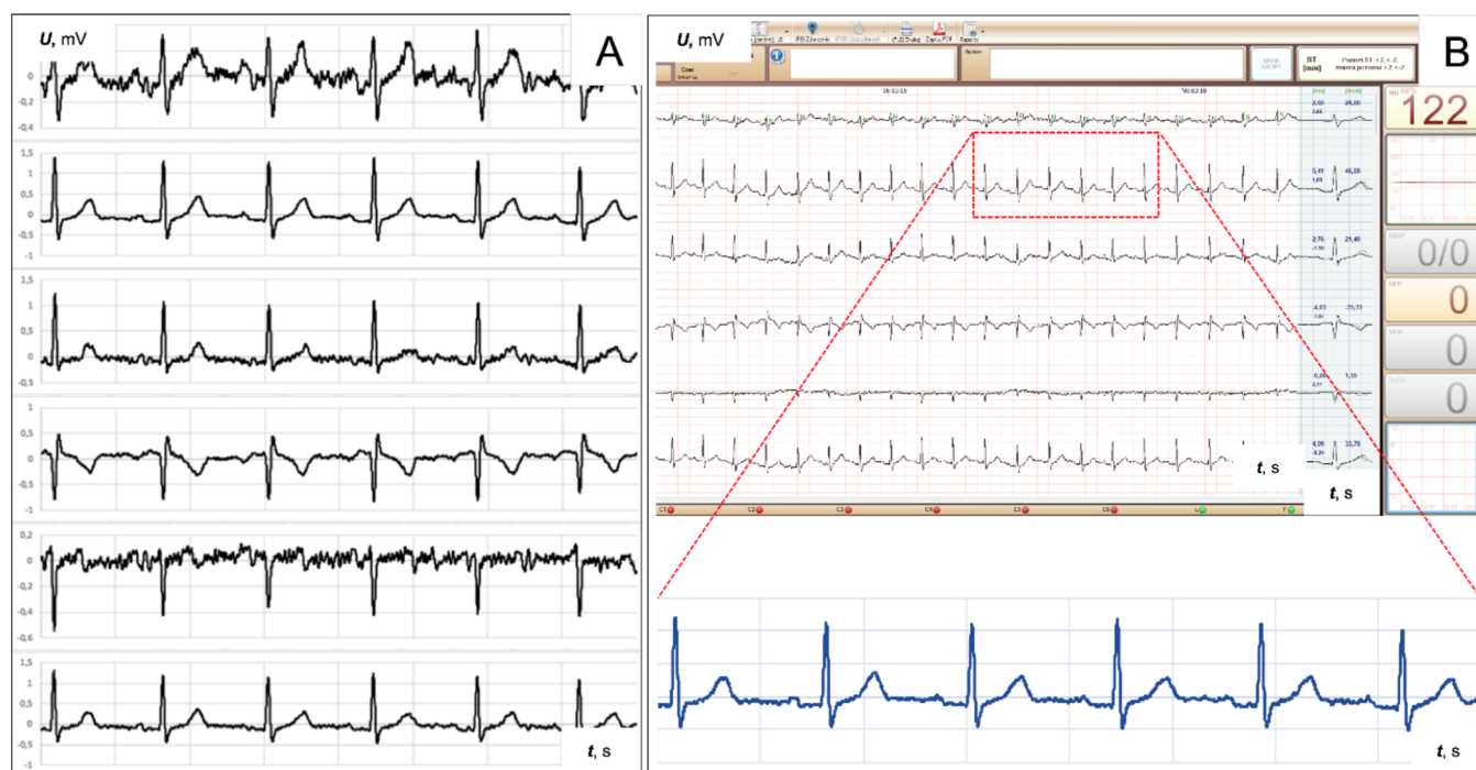
Figure 7. Six-lead ECG signals from the optimized version of the medical grade T-shirt using arrangement IV (from Figure 5), which was recorded during the stress test: (A) initial ECG tracing; (B) ECG tracing after 3 min of walking.
