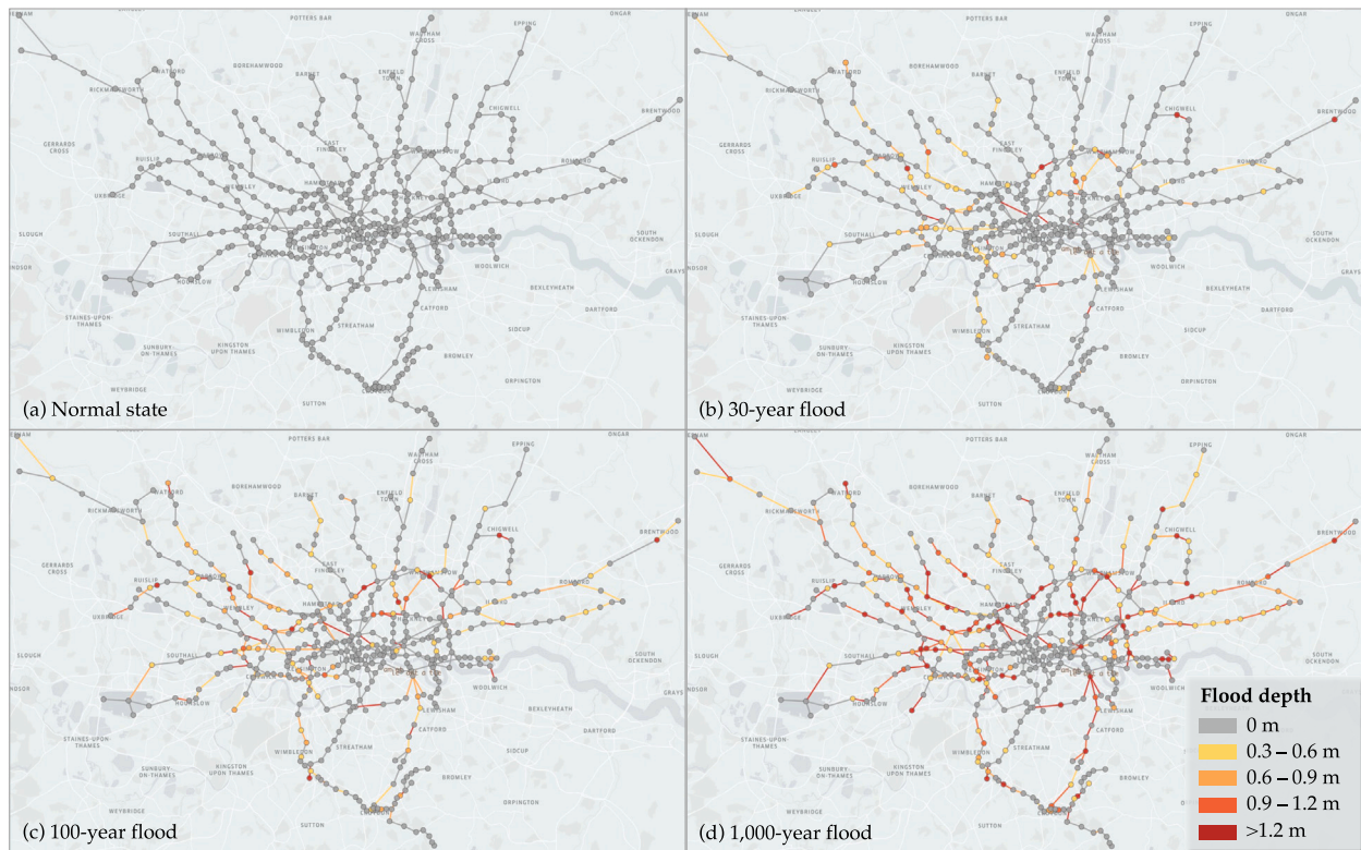
Fig. 9. Flooded stations and tracks of the London URTS with their flood depths (Bi et al., 2024).
