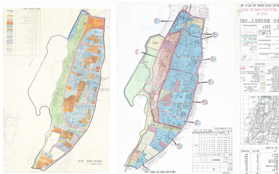
Figure 2: Approved sketch for altering Jaffa's coast to build the Slope Park with the existing plan on the left and the future plan on the right (the green area symbolising the park, the yellow a beach, and the blue and red a new residential area) (source: "Sketch for outline plan 2236 Midron Yaffo" by architect Avner Yashar, 1995; public domain; available from the Israel Planning Administration at https://mavat.iplan.gov.il/e2ee07f1-4bd5-4d86-880a-53a54aa60f85 )
