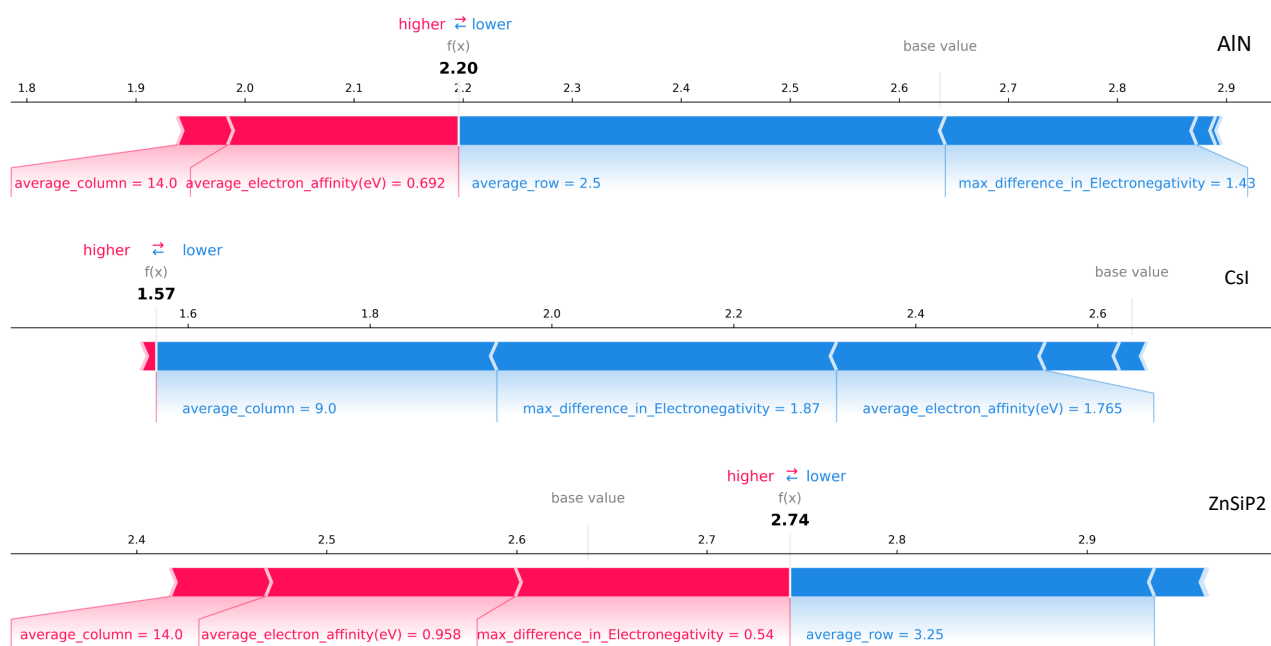
Fig. 7: Visualization of the Shapley values of the SVR model of compound AlN (top), CsI (middle), and ZnSiP 2 (bottom). Bars in red indicate this descriptor "pushes" to increase the prediction; bars in blue indicate this descriptor "pulls" to decrease the prediction. The base value represents the value that would be predicted when no feature is known for the current output, i.e., the mean prediction of the test set. Only descriptors with top contributions are annotated.
