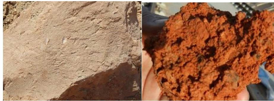
Figure 2. Comparison of expansive soil before and after encountering water.
