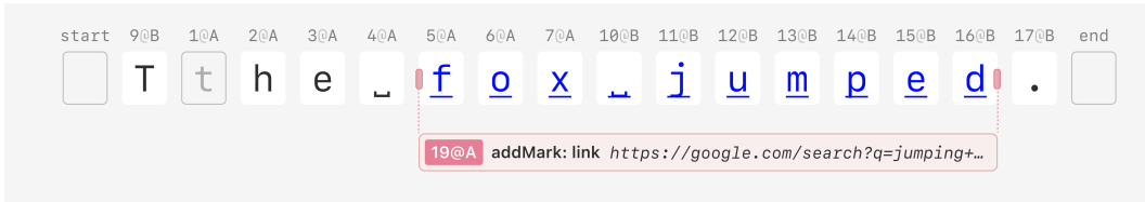
Fig. 5. Mark types can include additional metadata, such as a hyperlink. Note that unlike bold marks, which end on the character after the span, links end on the last character of the span. This approach prevents the link from growing when new text is appended.
