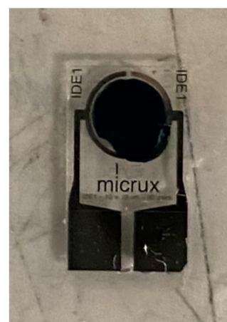
Fig. 4.54 (a) Schematic diagram of the Au-PB-Au interdigital electrode. (b) Digital images of the Au-PB-Au interdigitated electrode.
