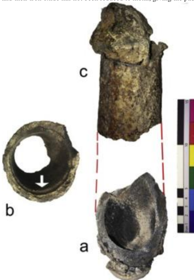
Fig. 1. Reconstructing a Chahak crucible with a. crucible base, featuring the base pad in the bottom; b. middle part of the crucible with slag line (due corrosion by molten slag) on the inner wall (marked by arrow), which is mostly where the crucibles break easily following by a blunt force to take the ingot out; and c. the upper part of the crucible with the lid still adhering to it.
