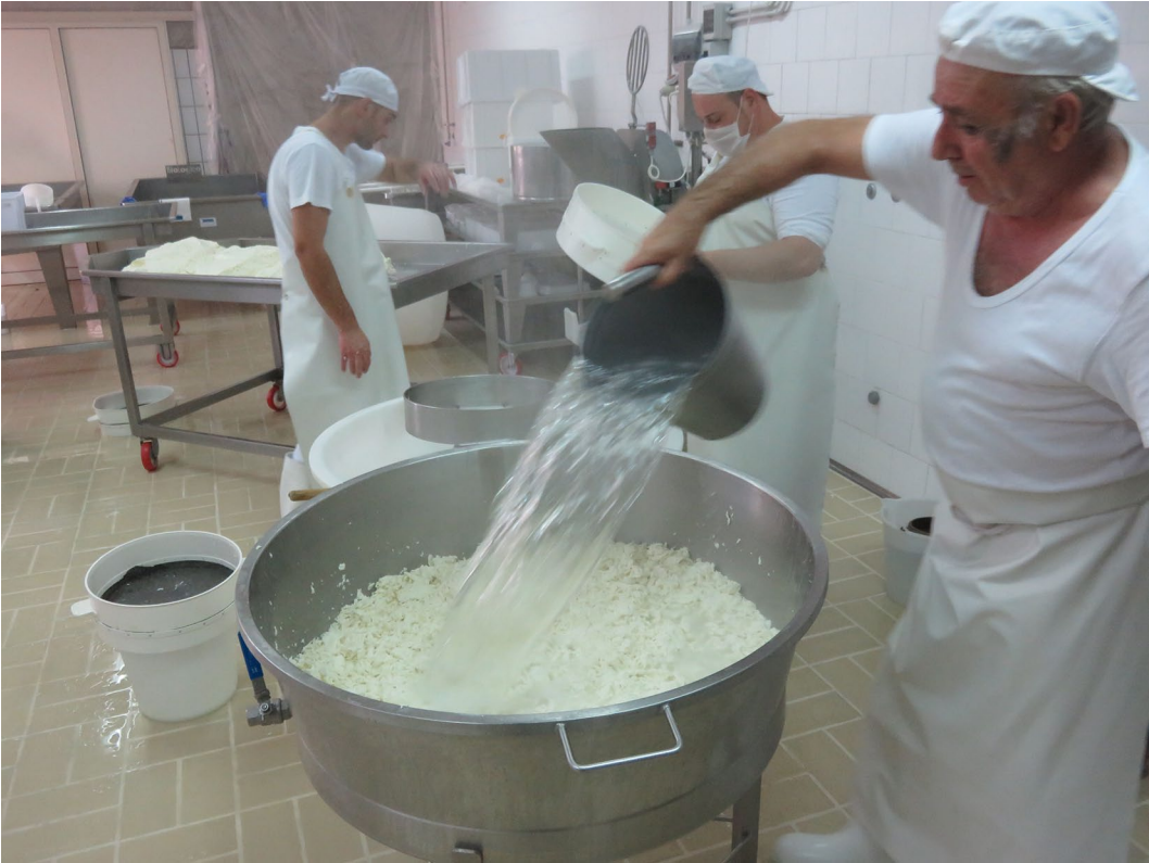
Figure 3. Using boiling water to process the paste in a mozzarella dairy near Naples. (photograph by the author).
