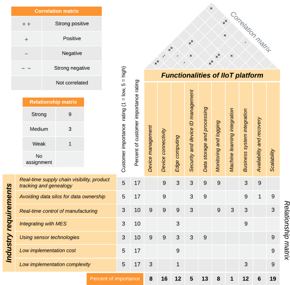
Fig. 5. The House of Quality – linking industry requirements with IIoT platform functionalities in Industry 4.0
