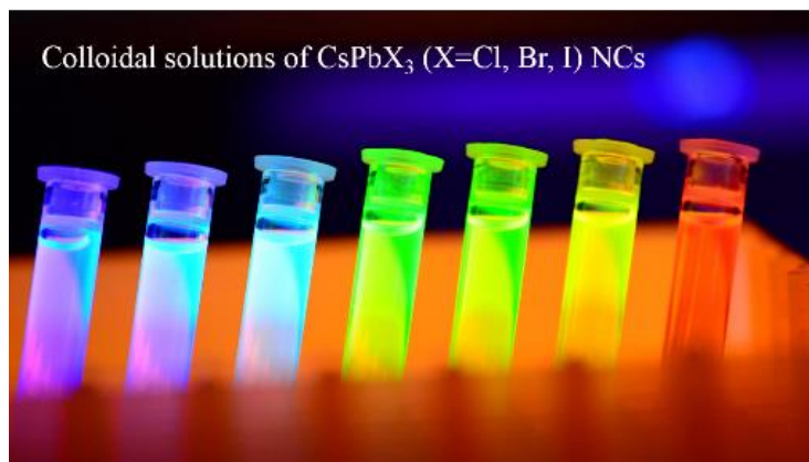
Figure 2. 6 Photograph of the colloidal dispersions of CsPbX 3 NCs with different halide (X=Cl, Br, and I) Reprint with permission under Creative Common Licence from Ref. 71 Copyright © 2021 American Chemical Society
