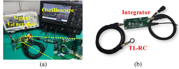
Fig. 16. Configuration of (a) DPT test rig and (b) TL-RC prototype.
