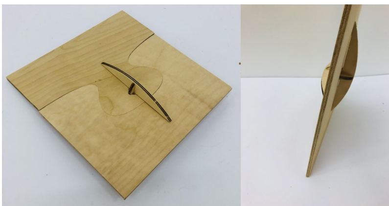
Figure 6. Key connection in 6mm plywood. Images by: Ana Gatóo
