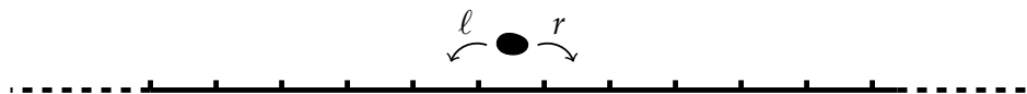
Figure 8. Simple random walk on an infinite, one-dimensional lattice in continuous time. The black blob indicates the current position of the random walker. The left and right hopping rates, labelled \ell and r respectively, are assumed to be homogeneous but not equal in general, thus leading to a net drift of the average position.
