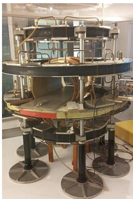
Figure 8. The original Aberdeen Mark 1 MRI scanner. Note how the patient is positioned between rather than through the magnet windings. Image taken in the Suttie Art Space in Aberdeen Royal Infirmary where the device has been on display since February 2016. AndyGaskell, CC BY-SA 4.0 < https://creativecommons.org/licenses/by-sa/4.0/ >, via Wikimedia Commons.
