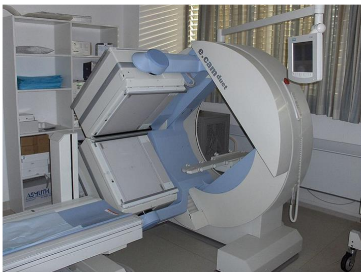
Figure 9. A dual-headed single-photon emission computed tomography (SPECT) camera circa 2006. User:Drahreg01 ( https://commons.wikimedia.org/wiki/File:SiemensEcamDuet.JPG ), „SiemensEcamDuet“, https://creativecommons.org/licenses/by-sa/3.0/legal code .
