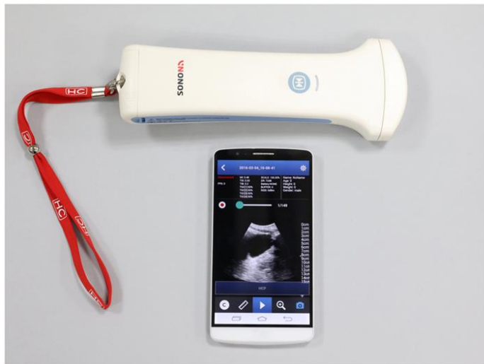
Figure 13. A pocket-sized ultrasound device. Images are displayed on a smartphone via a device-generated wireless connection. Under a Creative Commons (CC) license permission to publish this picture was obtained from HEALCERION, Seoul, Korea (S2 File). https://doi.org/10.1371/journal.pone.0185031.g001 .
