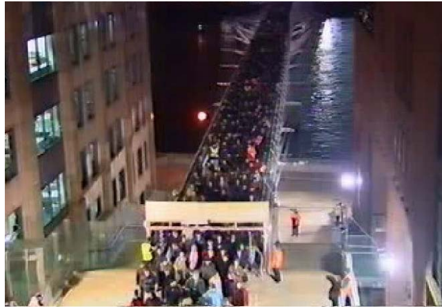
Figure 6: pedestrian acceptance tests demonstrated the success of the bridge modifications.
