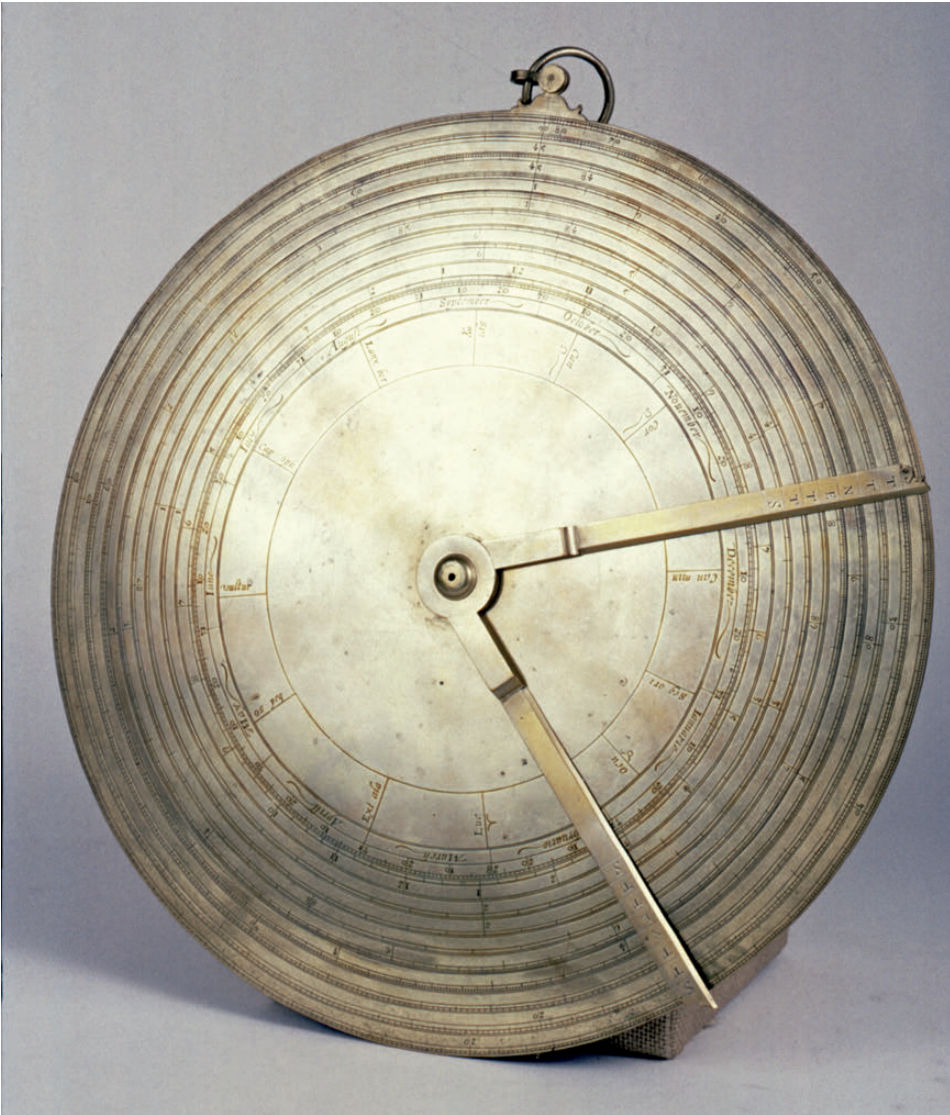
Figure 3. “Circles of proportion,” a circular logarithmic scale by Elias Allen to the design of William Oughtred, English, ca. 1635. As with a number of Allen’s instruments, XRF analysis of this object reveals a very high level of zinc in its brass alloy—in excess of 35%—an amount at the very upper limits achievable in the traditional “cementation” process of brass manufacture. How this brass was made, and where Allen sourced it from, remain open questions that cannot be answered without a much wider assessment of the brass used in the manufacture of 16th- and 17th-century European instruments. Wh.o833, Whipple Museum, Cambridge, UK. Reproduced with permission.
