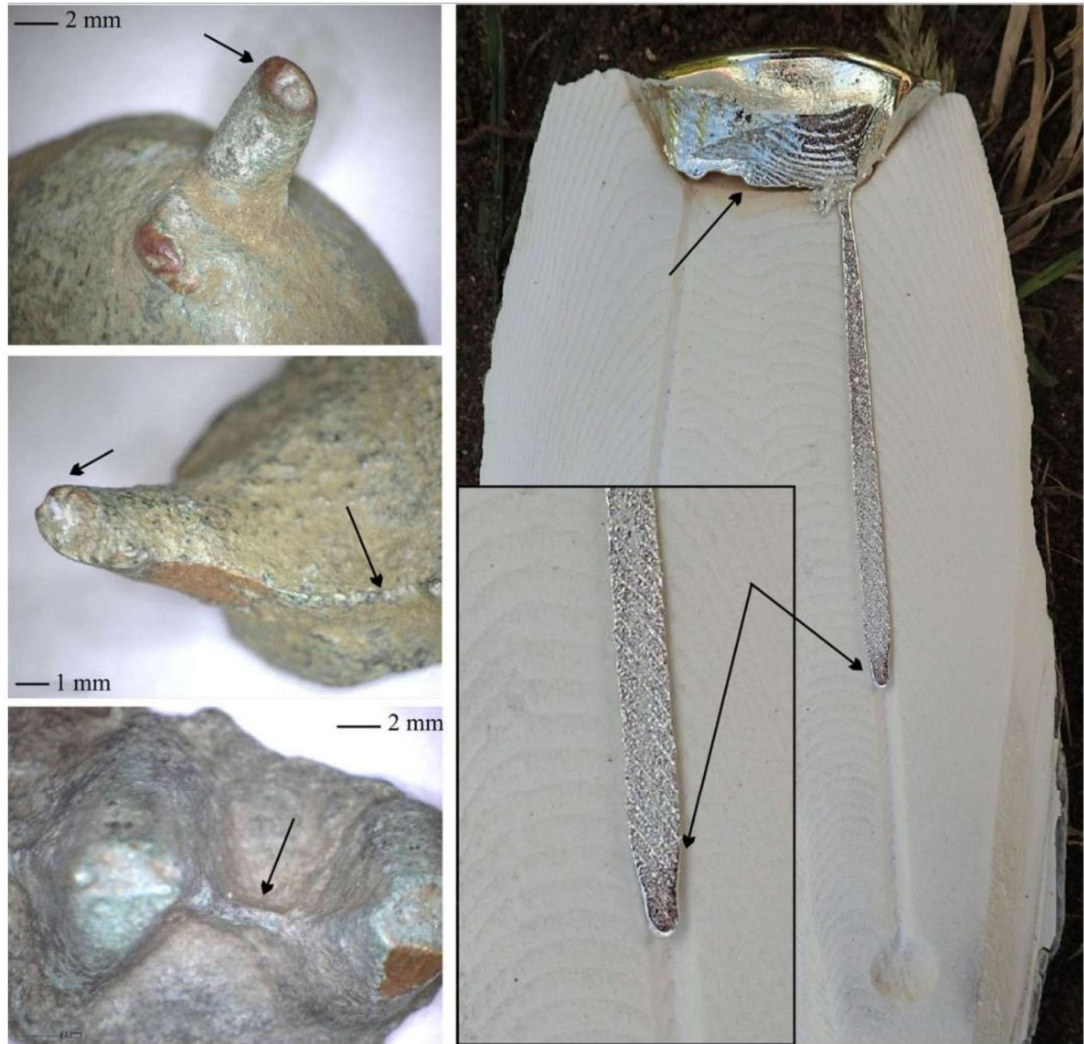
Figure 5 - Photomicrographs showing sprue ends from Rendlesham (left) compared to a modern failed casting experiment with flashing and a rounded end due to surface tension of the metal (right). Top left: EKE 022 1143 showing rounded end from failed casting. Middle left: RLM 013 0570 showing cut end from successful casting and flashing. Bottom left: RLM 013 0642 showing flashing. Right: results of a failed experimental session, showing the resulting rounded end of the metal within the cuttlefish mould (c 80 mm wide). Object photographs Copyright Eleanor Blakelock/Suffolk County Council Archaeological Service; experimental photograph Copyright Eleanor Blakelock.
