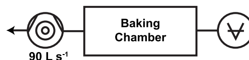
Fig. C.1. Schematic of the ultrahigh-vacuum test chamber, also used for initial baking of samples. Total pumping speed out of the sample chamber is approximately 90 L s -1 . N 2 pumping speed quoted. Pressure gauge is an Edwards Wide Range Gauge (WRG) [27].
