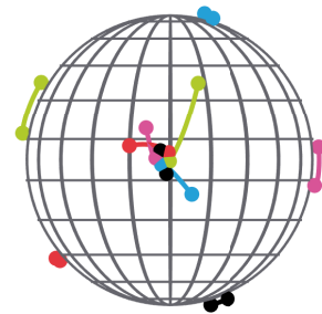
Fig. 3. The trajectories of five agents on \text{St}(2, 3) that are connected by the graph \mathcal{H}_5 . Each agent state is represented as an orthogonal pair of vectors on \mathcal{S}^2 . The agents are initially perturbed away from the equilibrium set \mathcal{Q}_{2,3} but ultimately end up close to it.
