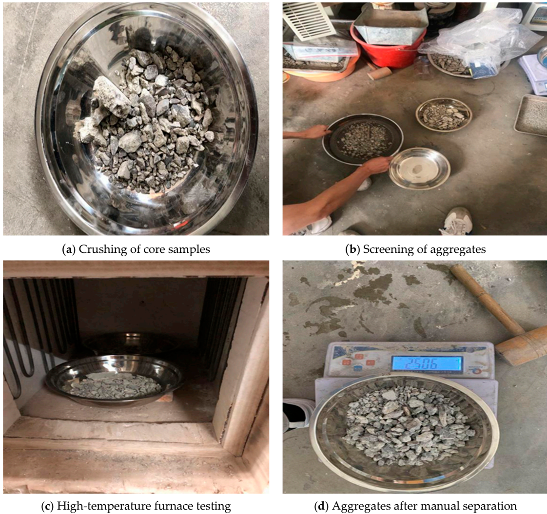
Figure 3. Experimental procedures for concrete aggregate testing.
