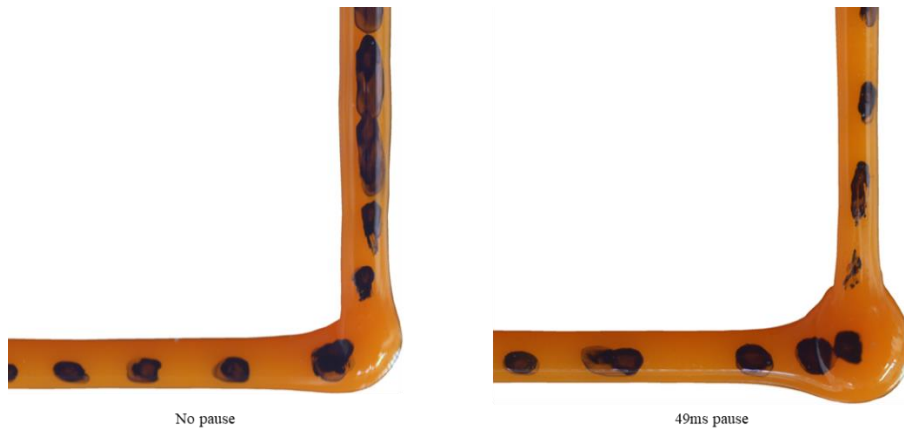
Figure 9.9 Effect of corner pause using standard machine and nozzle
