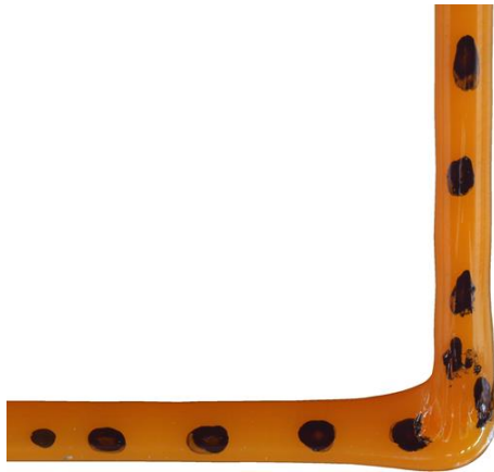
Figure 9.15 200°C and 10mm retraction with 49ms pause at corner
