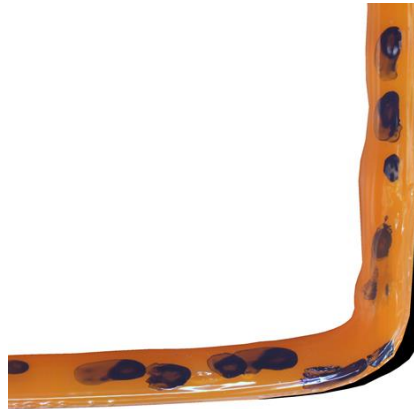
Figure 9.13 Effect of adding 5mm F10800 filament retraction during corner rotation
