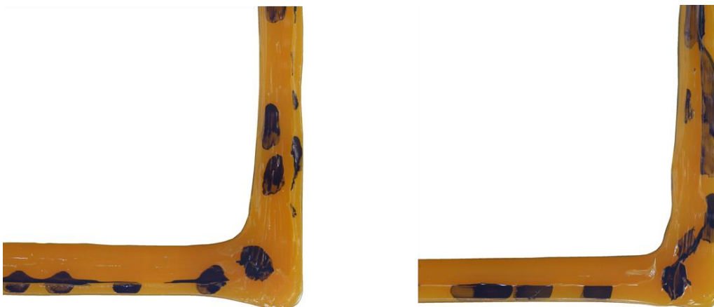
Figure 9.6 Single layer 90 degree corner using modified nozzle on 4-axis machine with wiper (F1800, left and F450, right)
