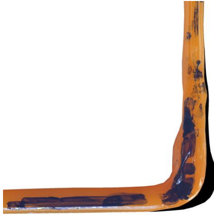
Figure 9.4 90 degree corner with reduced temperature (200°C) and extrusion factor (1)
