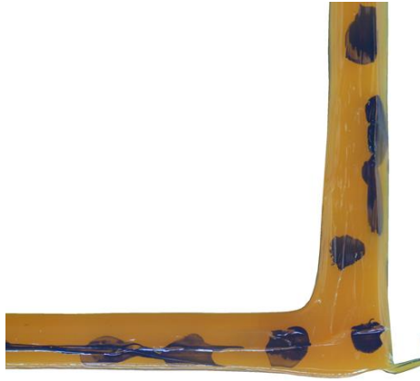
Figure 9.7 Single layer 90 degree corner using modified nozzle on 4-axis machine with straight wipe beyond corner (F450)
