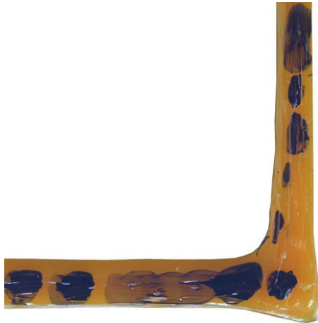
Figure 9.5 Single layer 90 degree corner using modified nozzle on 4-axis machine
