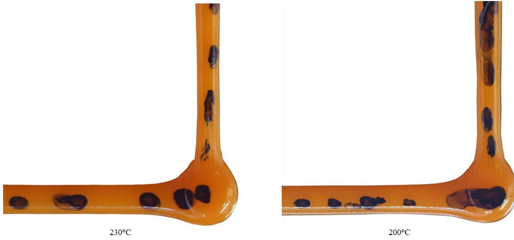
Figure 9.14 200°C and 230°C 90 degree corners using standard nozzle and machine with 49ms pause at corner
