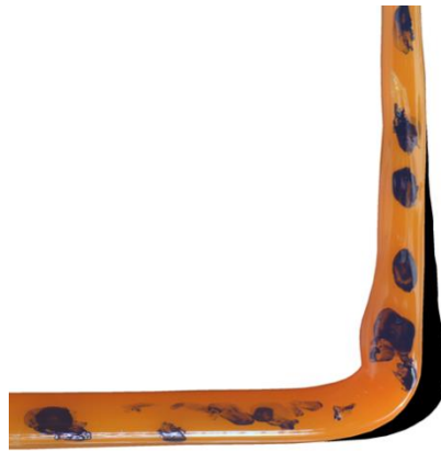
Figure 9.10 90 degree corner with rotational modified nozzle and optimised corner delay time
