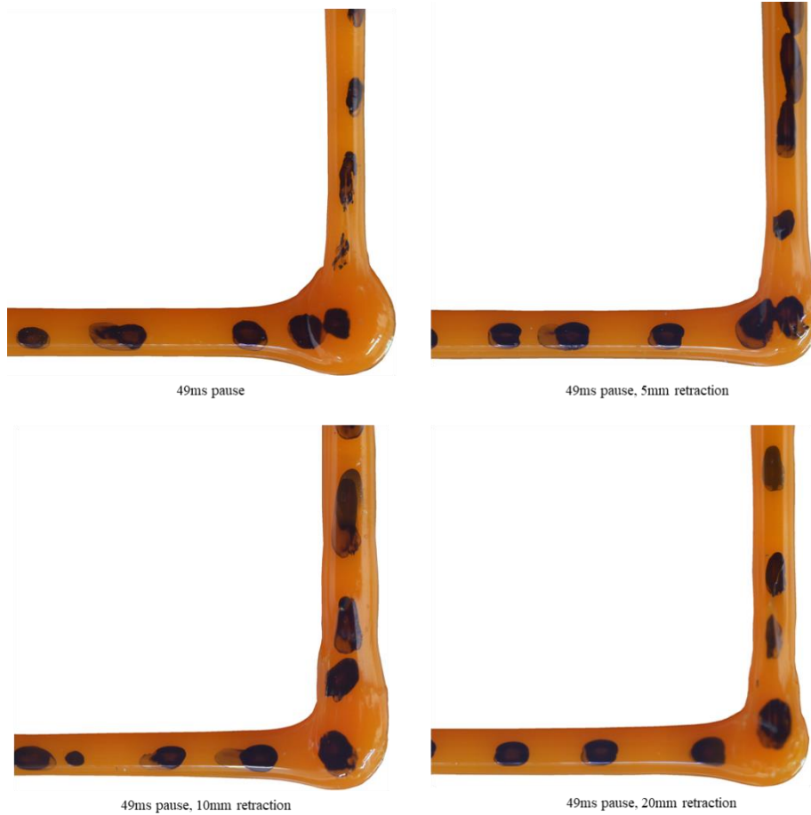
Figure 9.12 Effect of adding filament retraction during corner pauses
