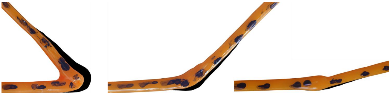
Figure 9.10 90 degree corner with rotational modified nozzle and optimised corner delay time
