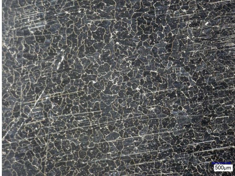
Fig. 1. Grains observed in the Co-27Cr-5Mo alloy after HIP and PST.
